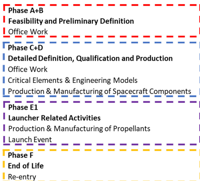
Fig. 5. System boundaries of a generic CubeSat mission.
